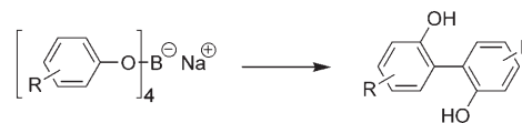
Scheme 6. Template-directed electrochemical synthesis of 2,2'-biphenols. Reagents: Pt electrodes, \text{CH}_3\text{CN} , 40°C, then hot water (60°C), citric acid.
